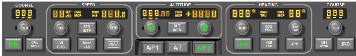
Image of Flamingo's Mode Control Panel (MCP)
